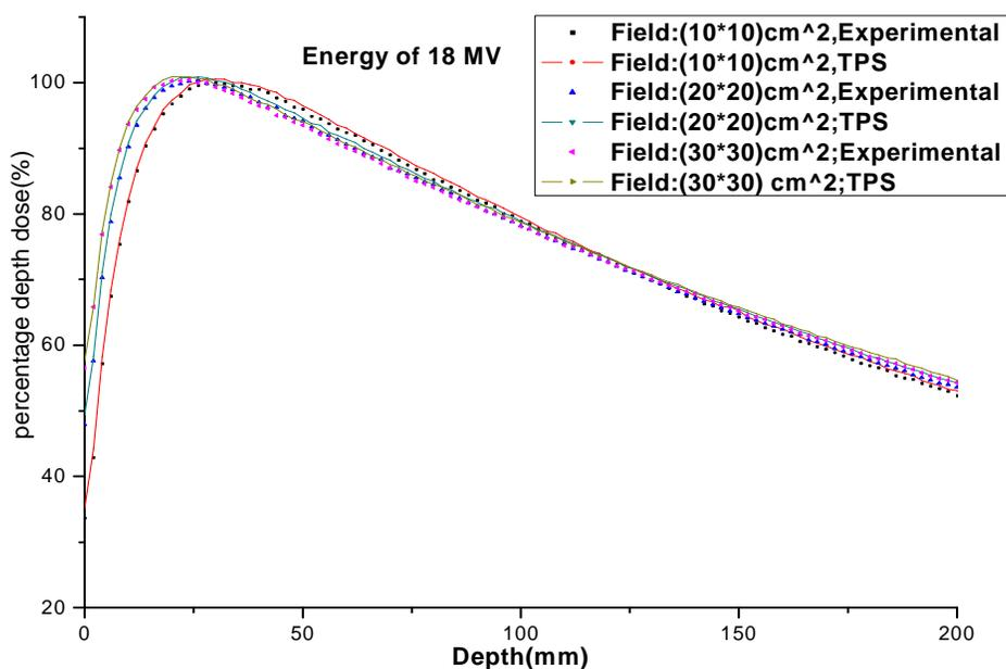
**Fig. 3. Comparison of measured and calculated results of percentage depth dose curves of the 18 MV photon beam for different field sizes**
