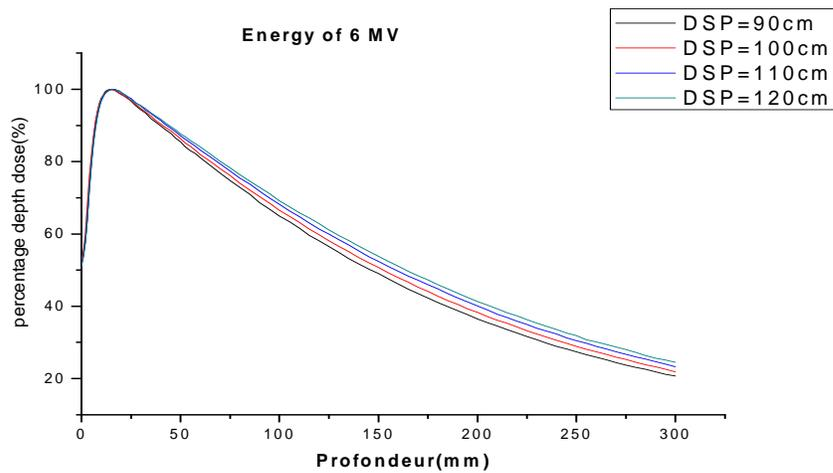
Fig. 8. Variation of percentage depth dose curves as a function of (SSD), for a 6 MV photon beam
