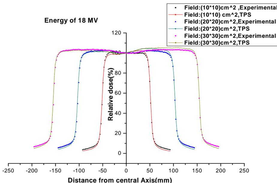
Fig. 5. Comparison of measured and calculated results of beam profiles of the 18 MV photon beam for different field sizes
