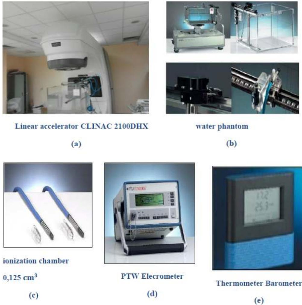
**Fig. 1. The devices used in this work**
