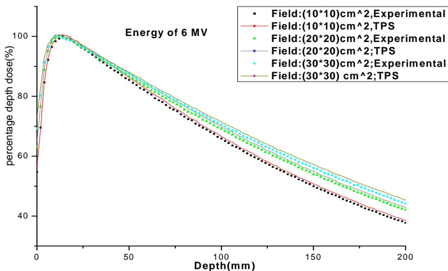
**Fig. 2. Comparison of measured and calculated results of percentage depth dose curves of the 6 MV photon beam for different field sizes**
