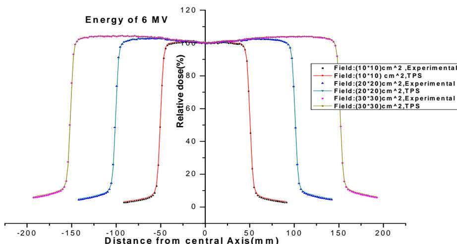
Fig. 4. Comparison of measured and calculated results of beam profiles of the 6 MV photon beam for different field sizes
