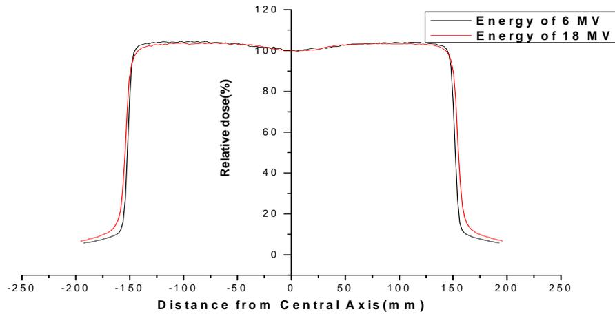
Fig. 7. Variation of the dose profile as a function of the energy
