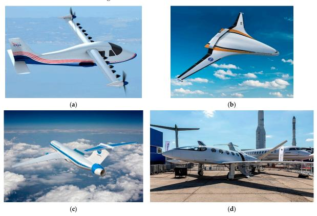
**Figure 16.** Disruptive configurations using DEP technologies: (a) NASA X-57; (b) NASA N-X3; (c) NASA STARC-ABL; (d) Eviation Alice/Matti Blume/CC BY-SA.
