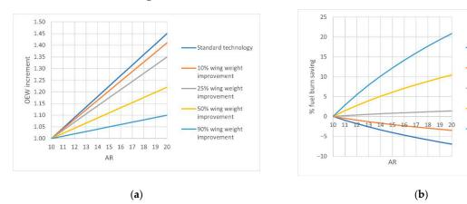
**Figure 30.** Example of potential weight increase and fuel burn variation due to aspect ratio variation: (a) change in operative empty weight; (b) change in fuel burn.
