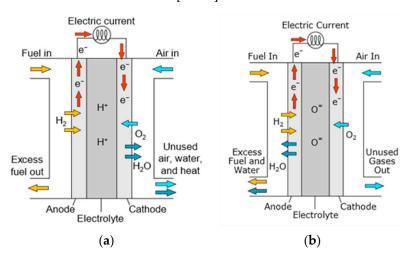
Figure 13. Scheme of two types of fuel cells: (a) PEM fuel cell; (b) SOFC fuel cell.
