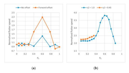
**Figure 37.** Normalised flutter speed: (a) for engine placement along the span for two values of chordwise offset; (b) in four-engine configuration with one engine fixed ( $\eta$ 2) and the other moving ( $\eta$ 1).
