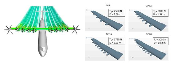
**Figure 24.** High-lift propeller on a typical 40-passenger regional turboprop wing, AR = 11.07, M = 0.15,  $Re = 7.6 \times 10^6$ , DEP 8, DEP 12, DEP16, and DEP 20 configurations,  $T_0$  is the thrust per propeller.
