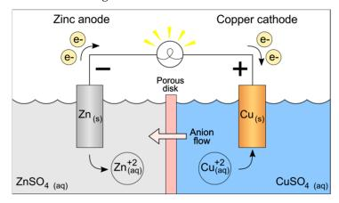
Figure 11. Working principle of a galvanic cell. CC BY-SA [29].
