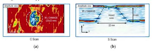
**Figure 31.** Low velocity impact damage: (a) typical peanut shape in the plane of the plate; (b) conical distribution of delamination through the thickness.
