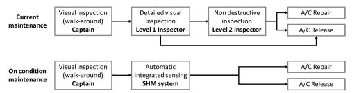
Figure 35. Possible maintenance approaches suited for aircraft operators.
