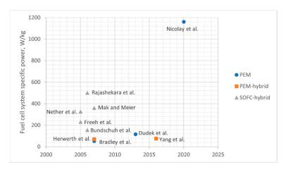
Figure 15. Specific power of fuel cells systems for aircraft applications.
