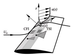
Figure 26. Transition mechanisms on a swept wing. Herbert.Oertel/CC BY-SA.
