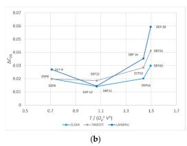
**Figure 25.** Effects of high-lift propellers on a typical 40-passenger regional turboprop wing, presented as difference values with respect to the unblown isolated wing, AR = 11.07, M = 0.15,  $Re = 7.6 \times 10^6$ , DEP 8, DEP 12, DEP16, and DEP 20 configurations: (a) lift coefficient change  $\Delta C_L$  at  $\alpha = 15^\circ$ ; (b) parasite drag coefficient change  $\Delta C_{D0}$ ; (c) pitching moment coefficient change  $\Delta C_{M0}$  at  $\alpha = 0^\circ$ .
