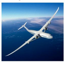
Figure 29. SUGAR Volt truss-braced wing aircraft concept.
