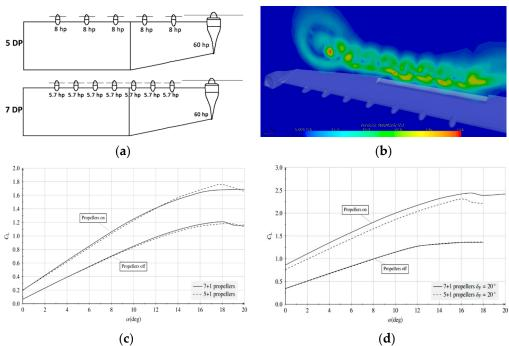
**Figure 23.** Tecnam P2006T wing simulated at M = 0.08, Re =  $3.3 \times 10^6$ , from Ref. [8]: (a) wing planform; (b) vorticity magnitude contour behind the wing; (c) lift coefficient in clean configuration; (d) lift coefficient in flapped configurations.
