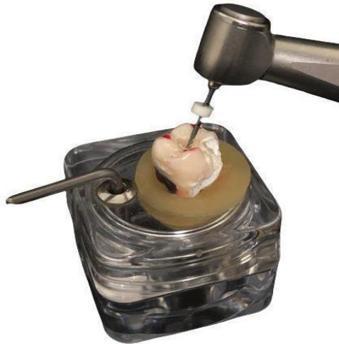
Fig. 1. Apparatus simulating the alveolar cavity
