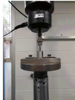
Fig. 3. Mechanical flexural test: A) Data of 2.4 and 1.3 (mm) thickness samples, fracture load 163 and 45 (N), respectively; Instron equipment used to perform the tests (FEM-UNICAMP)
