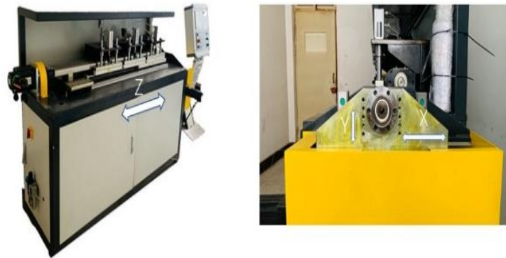
Fig. 9. Three axis movement direction of free bending equipment
