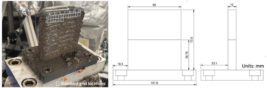
Figure 4. Illustration of an object made of LTT steel used in our experiments with an overlaid grid. The right panels show the dimensions of the object—which is 10 mm in thickness and 73.5(height) \times 65 mm in the face exposed to the neutron beam. The white boxes illustrate the footprint of the region being sampled (gauge volume) by the neutron beam. The overall object is mapped by stepping the stage one point at a time through the incident neutron beam. The successive steps can correspond to overlapped regions for a finer sampling grid. Depending on the size of the object and the beam-footprint, the total time to map the strains can be of the order of several hours. In our case, the gauge volume is about 5 \times 5 \times 5 \text{ mm}^3 and the object is stepped by 2.5 mm each time. Furthermore, we have used a thin sample (10 mm in depth dimension) in order to demonstrate the method on a 2D case.
